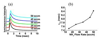
Fig.3 (a) The temporal evolution of PL intensity at the peak energy as a function of  $NH_3$  flow rate for the *a*-Si QD samples, (b) Carrier lifetime relevant to 1/e of the time-resolved PL maximum intensity as a function of  $NH_3$  flow rate.
