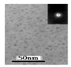
Fig.4. TEM image of a silicon in silicon nitride films grown with NH<sub>3</sub> flow rate is 35 sccm.
